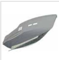
Naval architect, Guy Saillard, has applied his vast experience in designing trawlers, to design the hull lines to carry a full load of 32 tonnes, while reducing drag and fuel consumption to a minimum.
